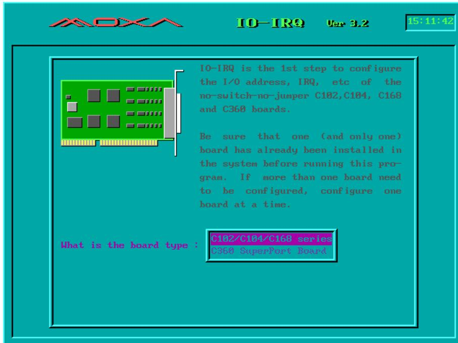
Choose the board type "**C102/C104/C168 series**" and press the Enter button, the following picture appears on the screen:
