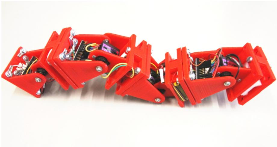
Prototype with 4 modules in pitching configuration.
