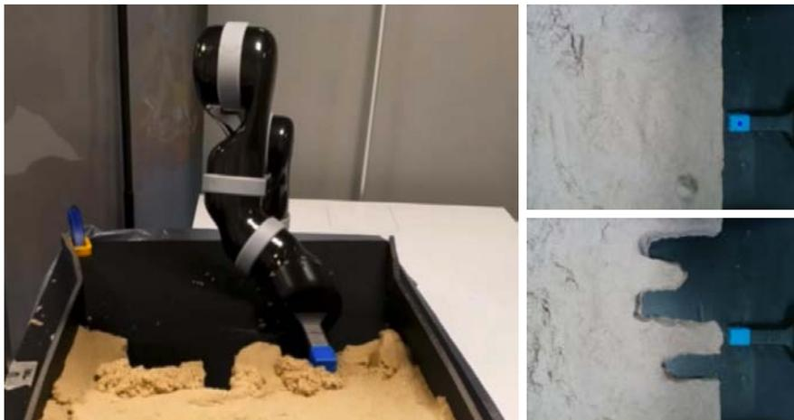
Figure 3.1.: The shape servoing task from [6]. The left image depicts the setup with the robot actively moulding the material with the tool (blue). The top right image shows the initial shape of the sand while a goal shape is depicted in the bottom right image.
