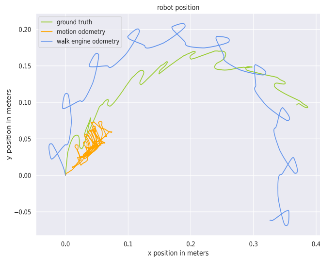
Figure 20: The walk engine and motion odometry plotted against the ground truth from simulation data. The base link of the walk engine odometry and the ground truth show sinusoidal movement due to the robot’s walking pattern. The motion odometry performs very badly as the double support phases are detected without regard to the actual step taken, as described in Section 4.4.1. However, it works for model-based walk engine odometry.
