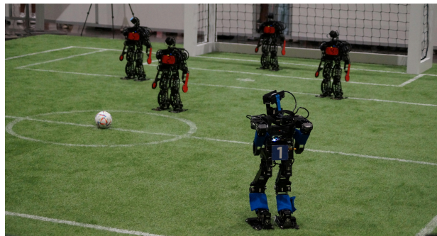
Figure 1: Robots of two different teams during the RoboCup 2023 in Bordeaux. They need to enter the playing field autonomously and position themselves for the kick-off. Source: [Bit24]
