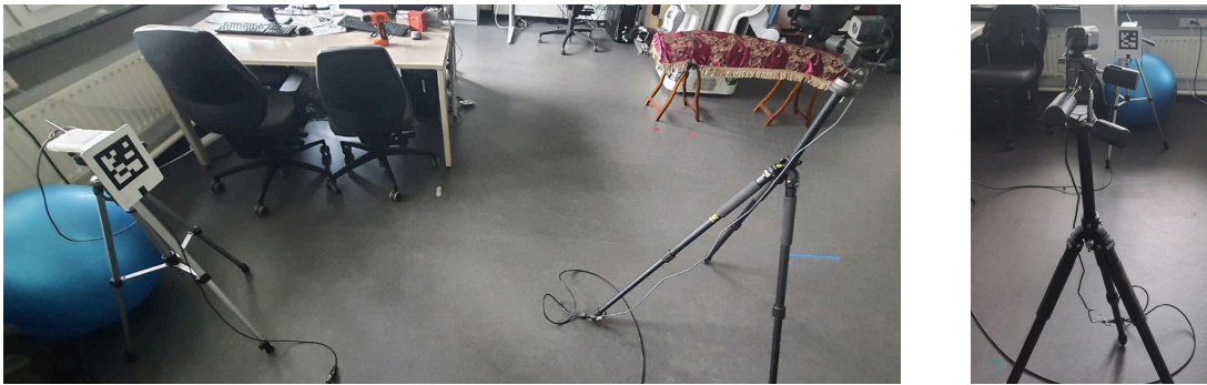
Figure 5.4: Setup with secondary webcam, Kinect's location is also measured through AprilTag .
