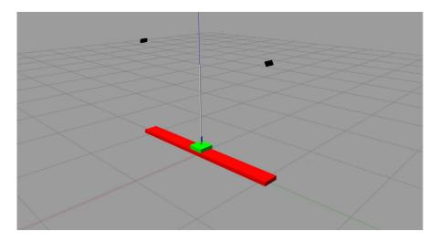
Figure 2.8: Gazebo screenshot of the x-y-slider setup
