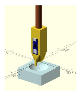
Figure 2.1: Pin-in-hole concept of the spherical joint connector. Top view angle
