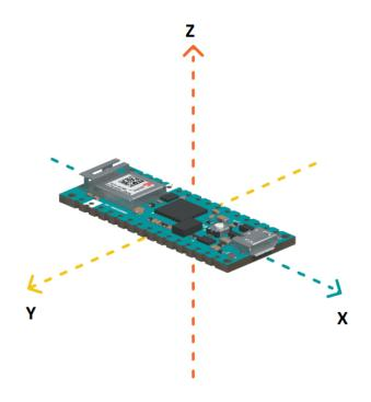
Figure 2.7: Schematic of the Arduino Nano 33 loT and the axes of its IMU [17]
