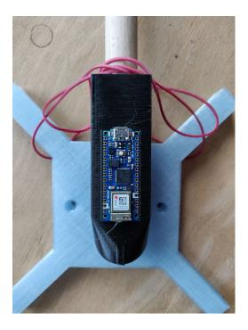
Figure 2.3: Laboratory shot of the IMU and the winged socket.
