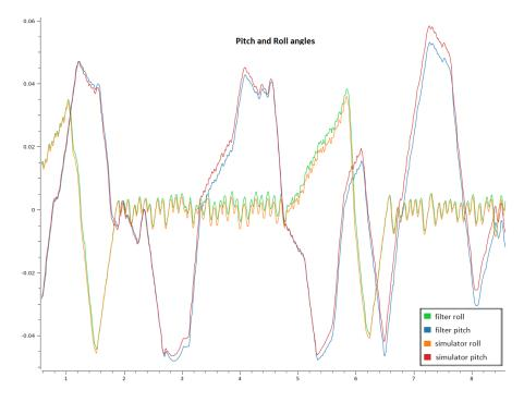
Figure 3.11: Roll and pitch angle calculated by the filter based on IMU data and true angle provided by the simulator
