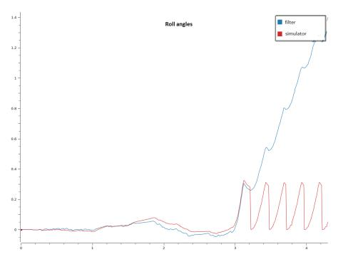
Figure 3.9: Roll angle calculated by the filter based on IMU data and true angle provided by the simulator
