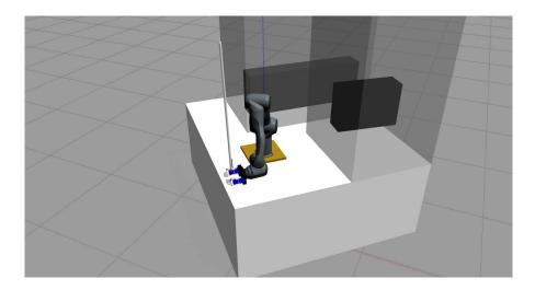
Figure 2.9: Gazebo screenshot of the simulation setup using the Diana7 model.
