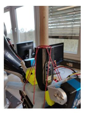
Figure 2.4: Close up laboratory shot of pole held in place by rubber bands
