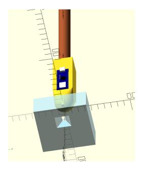
Figure 2.2: Pin-in-hole concept of the spherical joint connector. Bottom view angle
