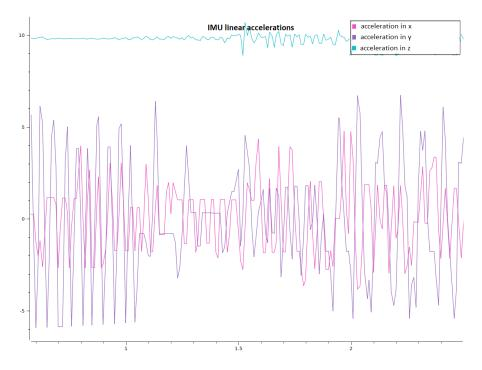
Figure 3.12: Linear accelerations measured by the IMU with reduced y-direction acceleration due to smaller parameter  $p_y$
