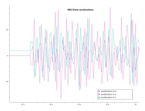
Figure 3.17: Linear accelerations measured by the IMU during simulation with a robotic arm
