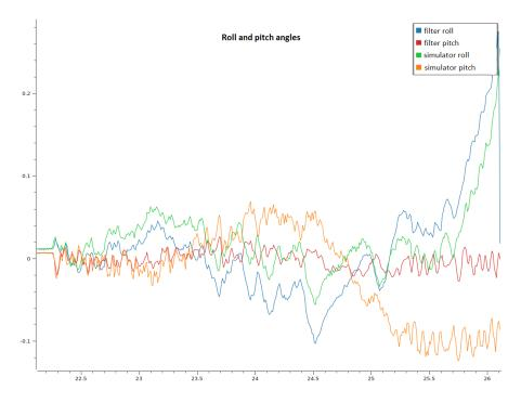
Figure 3.18: Comparison of pitch and roll angles provided by the filter and the simulator during simulation with a robotic arm
