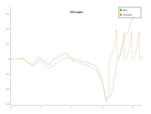
Figure 3.8: Pitch angle calculated by the filter based on IMU data and true angle provided by the simulator
