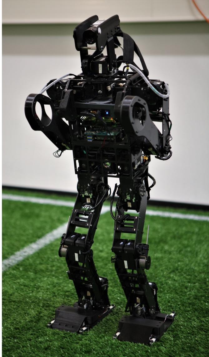
Figure 2.7: A humanoid Wolfgang-OP robot from the Hamburg Bit-Bots. Image used with permission of the owner.
