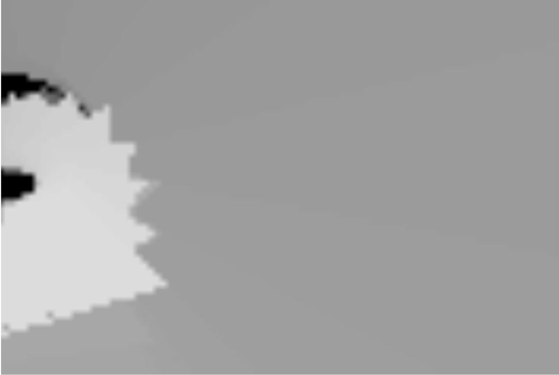
Figure 5.6: An example Motion History Image feature map before being processed by the CNN. The recently visible regions can be clearly seen in the bright part of the feature map, while unseen regions are black.
