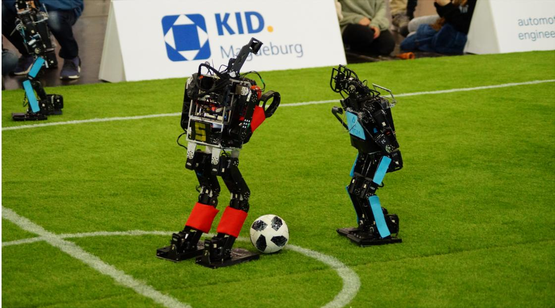
Figure 2.3: Three robots competing in the Humanoid Kid Size League. The Hamburg Bit-Bots in red use their Wolfgang-OP robot while Team Rhoban in blue plays with their SigmaBan robot platform. The differences in regard to e.g. size and proportions can be clearly seen.
