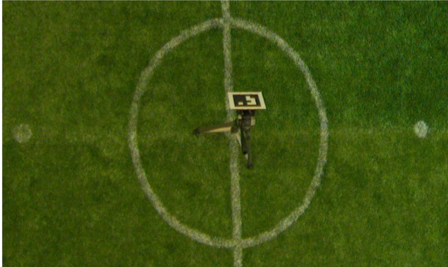
Figure 5.1: The setup to evaluate the orientation accuracy of the AprilTag Detection System. The AprilTag is mounted on a tripod in the middle of the field and tilted away from the ceiling camera. In this case it is tilted away 60 degrees. The image is taken from the ceiling camera.
