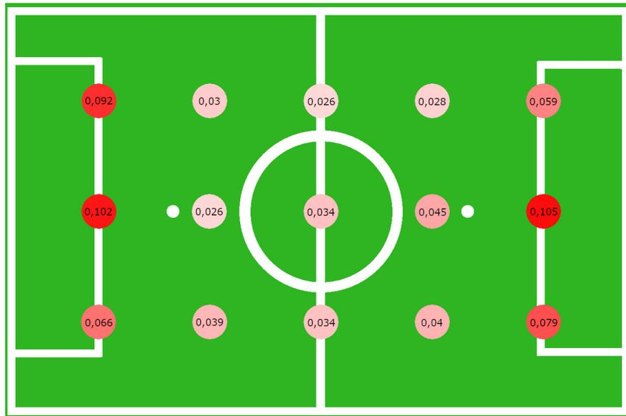
Figure 5.2: Average distance in meters of the detected 3D position to the real 3D position of a 16h5 AprilTag at each of the 15 positions on the field.
