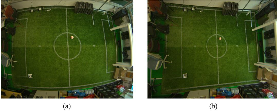
Figure 3.4: (a) shows the original image taken by the camera which is distorted and (b) shows the image after it was rectified.
