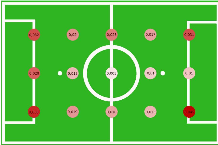
Figure 5.8: Average error in meters of the predicted ball position at 15 points on the field.
