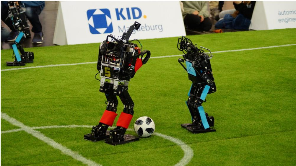
Figure 2.1.: Two robots in the Humanoid Kid Size League. On the left, the Wolfgang-OP used by the Hamburg Bit-Bots, on the right the SigmaBan Platform used by Team Rhoban. Differences between the robots in the Humanoid League are clearly visible. (Image used with permission of the owner.)
