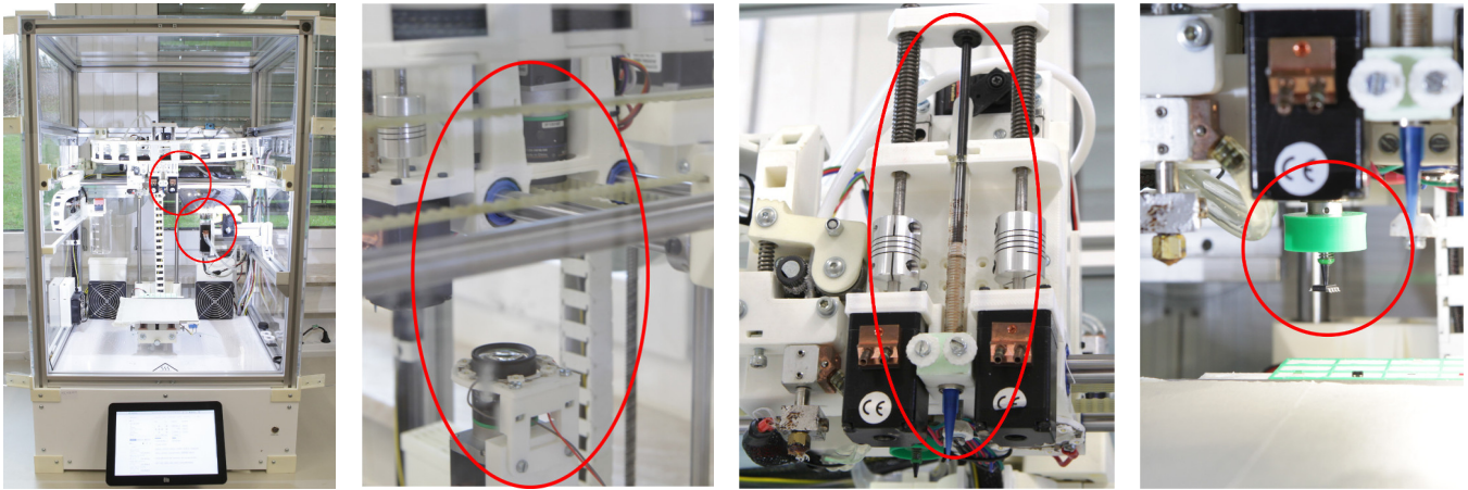
Fig. 3. Hardware setup used to print objects with integrated electronics. From left to right: a : modified RepRap Industrial printer, equipped with b : two cameras for component handling and process monitoring, one mounted at the printhead, one next to the printed bed c : a screw-driven conductive paste extruder and d : a rotating vacuum gripper for automatic component placement.
