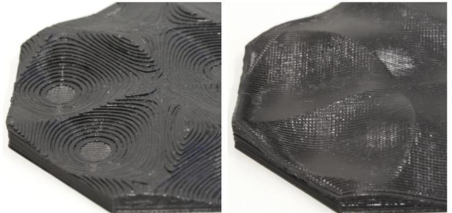
Fig. 2. FDM 3D-printed relief. **Left:** traditional slicing showing strong stair-stepping artifacts, **Right:** nonplanar slicing with smooth upper surface.
