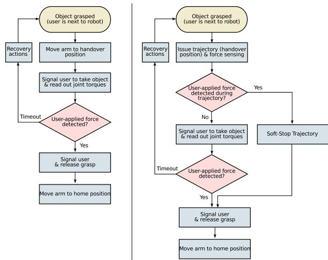
Fig. 2. (below) Flowchart of the handover controller (left): stationary robot arm, (right) in-motion handover. Here, the robot is switched to a soft-stop trajectory as soon as user interaction is detected.
