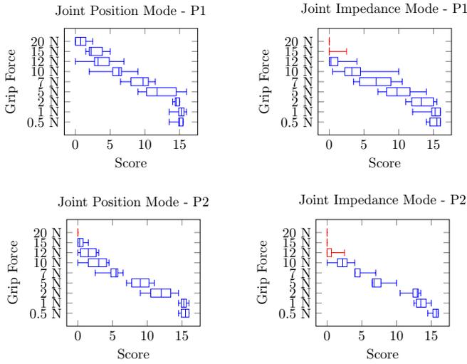
Fig. 3. User scores of handover force-threshold (“grip force”) versus object weight in four different robot control modes. From top-left to bottom right: (a) stiff robot, horizontal gripper orientation, (b) compliant robot, horizontal gripper, (c) stiff robot, vertical gripper, (d) compliant robot, vertical gripper. While higher force thresholds ensure a more reliable operation, users clearly prefer low interaction forces.
