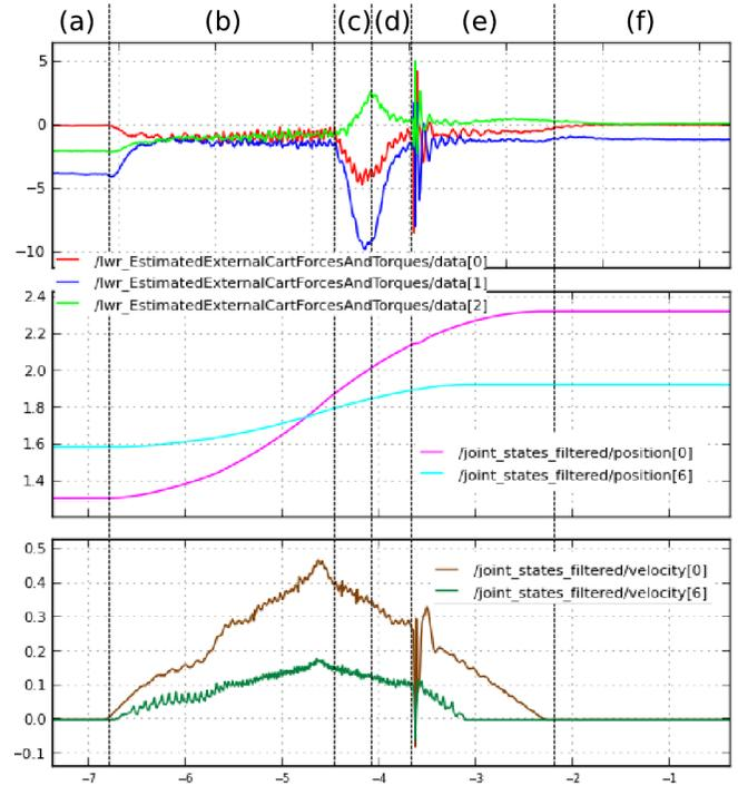
Fig. 4. In-motion object handover (LBR4+): (above) Measured external tool forces ( $F_x, F_y, F_z$ ); (middle) robot joint positions ( $\theta_0, \theta_6$ ); (lower) corresponding joint velocities. The annotation indicates the handover phases: (a): robot idle, (b): arm motion towards the user, (c): user touches and grasps the object, (d): gripper opens (and forces decrease), (e): arm stops, (f): robot stopped.
