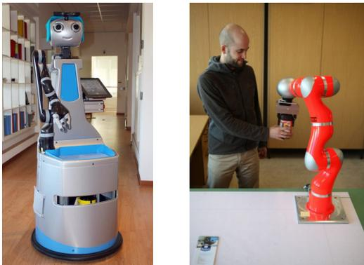
Fig. 1. The two robot systems used for the experiments: The *Domestic Robot* service robot designed for elderly care uses the Kinova Jaco arm (left). Our work cell setup with the KuKA LBR-4 in a robot-to-human handover task, shown with vertical gripper orientation (right). Our algorithm uses force and tactile sensor data to detect when to release the grasp.
