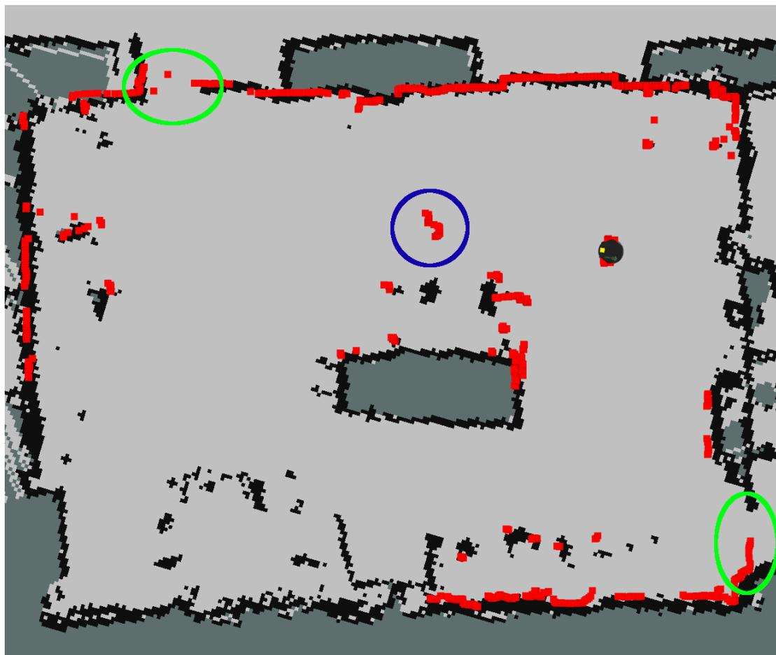
FIGURE 2.3: This is an example of how uncertainty plays a role in localization. The figure is very similar to figure 2.2, but signified by the blue circle there are measurements created by the laser range finder that do not fit to the map. The reason in this case was simply that a person was standing there. The green circles show doors that were opened when the map was created, but are now either closed or in a different position.
