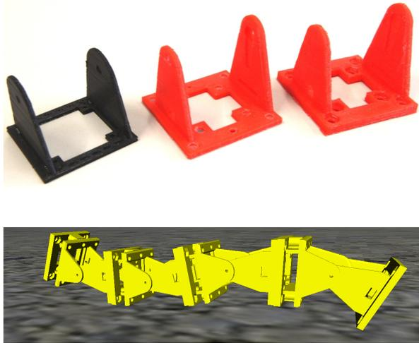
**Figure 1 – Upper:** Evolution of the robot design. Three versions of the lower module. Note the increased wall thickness in the second generation and improved magnet slots in the third generation. **Lower:** Simulation of mechanical assembly and locomotion in the OpenRAVE framework.
