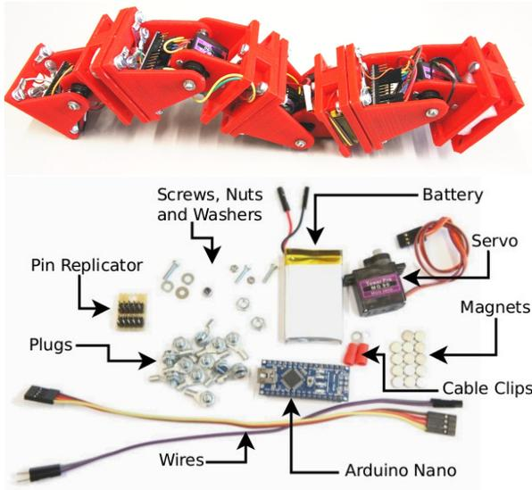
**Figure 3 – Upper:** Assembled robot with 4 modules in all-pitch configuration. **Lower:** Standard components of one PMR module. One servo motor and one Arduino board are needed for each module; batteries are optional but at least one battery is needed for a whole robot.
