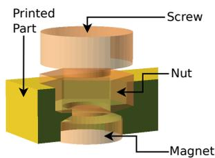
**Figure 5 –** Cross section of one magnetic connector. The magnet is glued into the narrowing slot, the screw/nut is fixed in its slot by magnetic force only.
