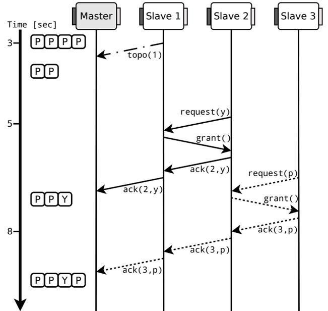
**Figure 8** – Sequence of the handshaking protocol to handle the changes in topology as illustrated in Figure 7. The master module stores the current topology. Disconnecting the last two modules in second 3 causes the last remaining slave module, slave 1, to send a topology update to the master. Reattached module slave 2 connects in yaw orientation at second 5 and slave 3 respectively in pitch orientation.
