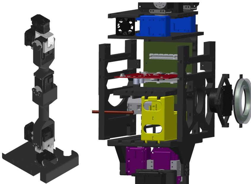
**Fig. 2:** CAD model of the leg (**left**) and explosion view of the torso (**right**). Note the additional shoulder servos (blue) and the new waist joint (purple). The two batteries (yellow, only one shown) are inserted from left and locked by a bolt (brown) which fits into a bayonet socket. The powerboard (red) and motor controller board (not shown) are directly plugged into the backbone board (green) and locked by a side plate (not shown).
