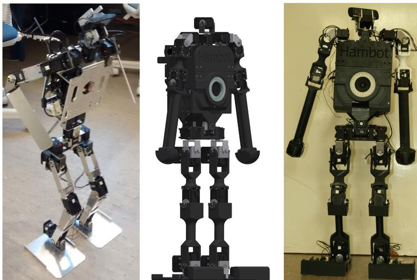
**Fig. 1:** Prototypes of GOAL (**left**) and Hambot (**right**). CAD model of Hambot (**center**).
