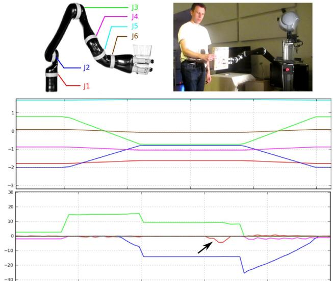
Fig. 4. Force controller handover with the Kinova Jaco arm. The robot arm and its joints (J1..J6) (top-left), a photo during handover-operation (top-right), measured arm joint-trajectory [rad] (middle) and joint-efforts [N] (bottom) during handover operation. In this experiment, handover was triggered by a force threshold on J1 (red line), the arrow marks the force that triggers release.
