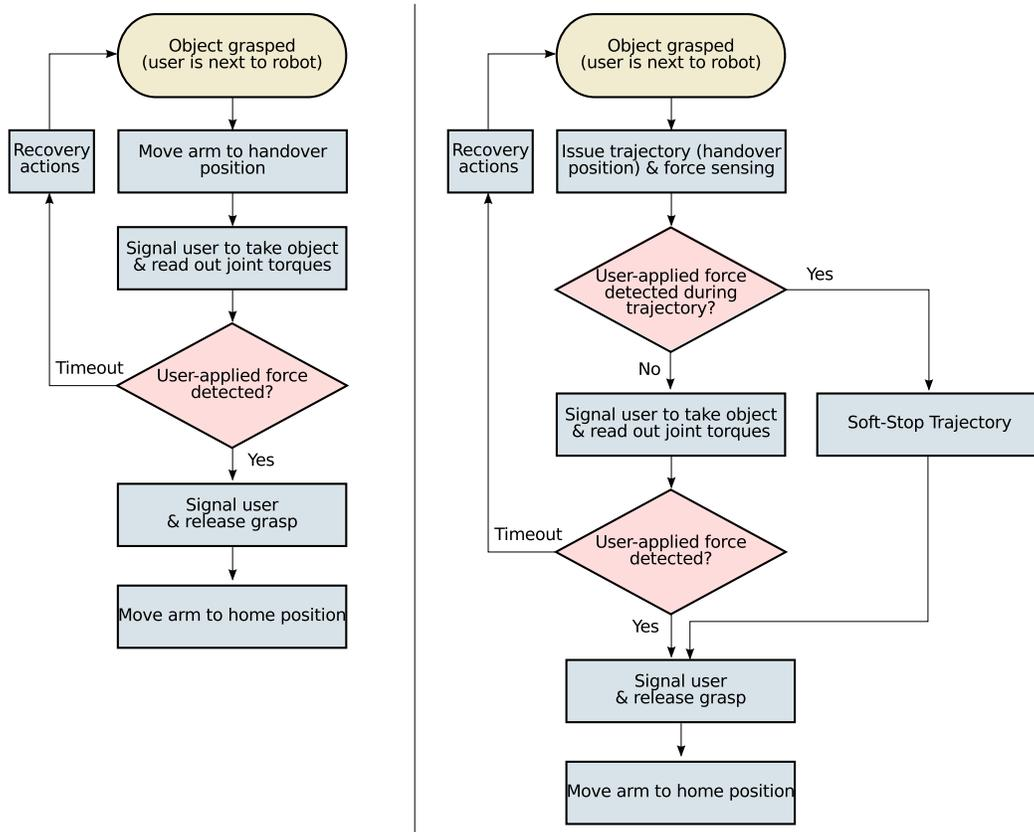
Fig. 3. Simplified state-machine diagram of the two handover controller modes. Left: the arm moves to the handover position and detects when the user applies force to the grasped object. Right: in this mode the force detection is already active during the trajectory execution. This operation mode required support in the ROS-node for trajectory control.
