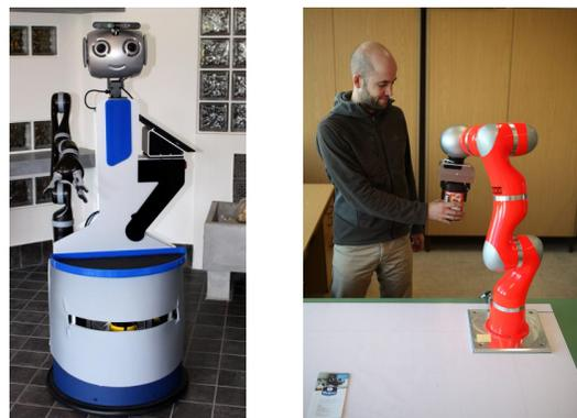
Fig. 1. The two robot systems used for the experiments: The mobile service robot (left) and an the work cell setup performing a robot-to-human handover task (right). Force-sensing is used to detect when to release the grasp.
