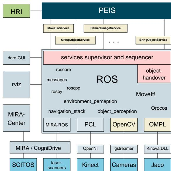
Fig. 2. The software architecture of the domestic robot platform and the planning components: The robot software is based on ROS and provides interfaces to the MIRA/Cognidrive navigation software and the PEIS ambient intelligence framework. The handover controller relies on MoveIt! and OMPL for motion planning, and OpenCV for perception.
