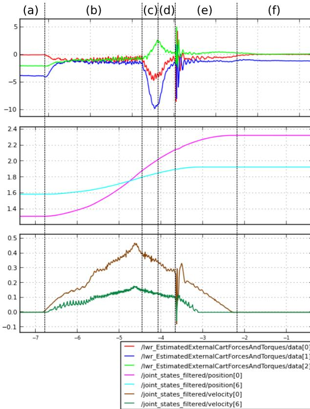
Fig. 8. In-motion-handover: The Cartesian end effector forces [N] (top), the joint position [rad] (middle) and joint velocity [rad/s] during the handover procedure. The different phases of the handover process can be seen:
