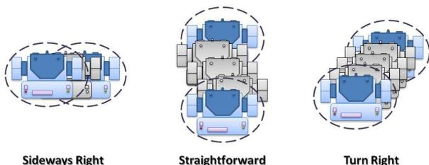
**Figure 3:** Different motion actions of the humanoid robot by using a cylinder model.
