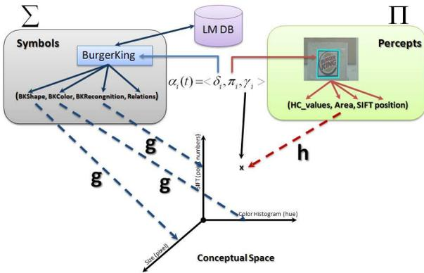
**Figure 2:** The anchoring process for a landmark between its symbolic and perceptual data.
