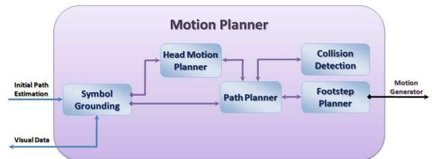
**Figure 1:** The architecture of the HOAP-2 humanoid robot motion planner.
