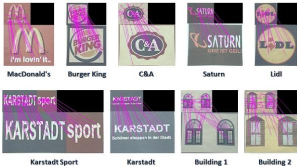
Figure 8. The matching between the calculated SIFT descriptors of the processed images and those of the stored landmarks in the knowledge base.
