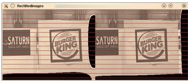
Figure 2. The resulting rectified image of the stereo pair.
