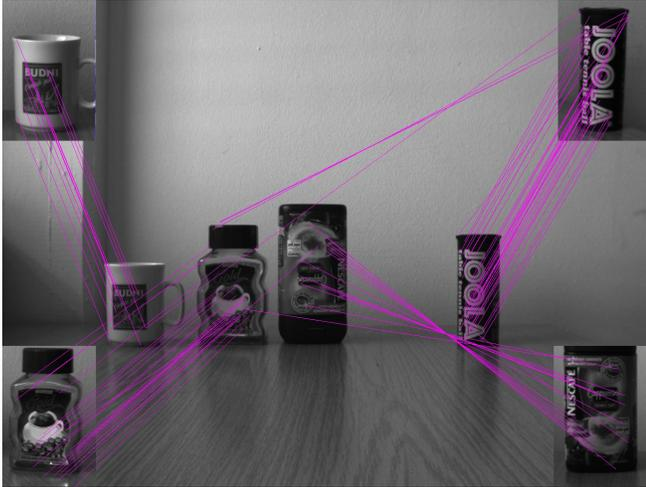
Fig. 5. This images shows a table scene with detected objects and the matches between features of the model and the corresponding ones of the image. Some mismatches occur but due to the high amount of correct matches these can be filtered out.
