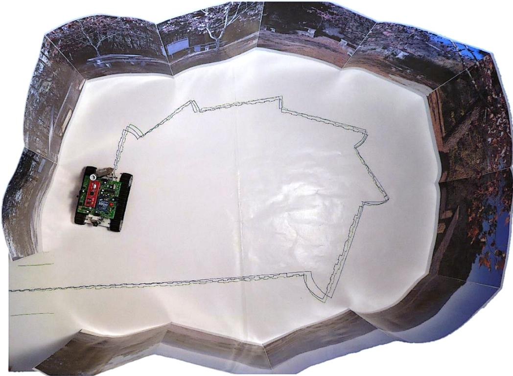
Figure 6.2.: LIZARD in its experimental environment. Figure adapted from Mendes et al. (2008). The blue line depicts the path taught during a supervised learning stage. The other lines result from autonomous runs of the robot guided by its memory.
