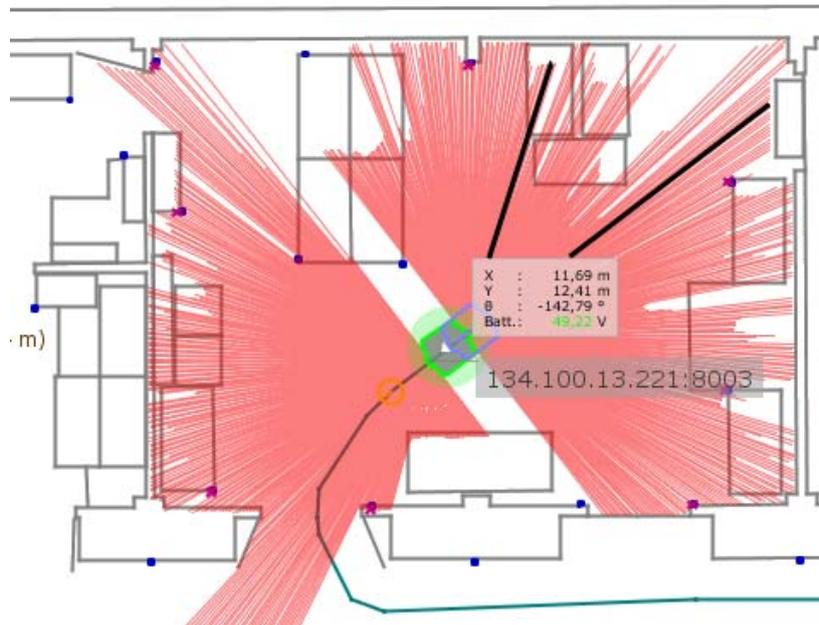
Figure 8.2.: A laser range scan of the robot standing in the laboratory. Each red line shows a laser beam and its distance of reflection.
