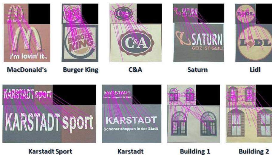
Figure 8.16: The matching between the calculated SIFT descriptors of the processed images and those of the stored landmarks in the knowledge base.
