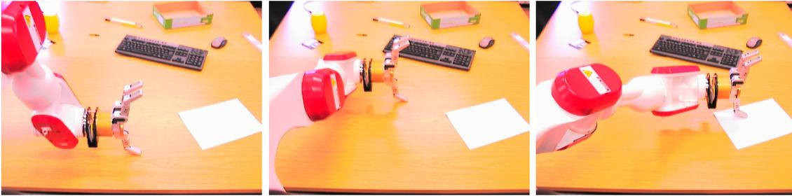
(a) The robot touches the table top to self-calibrate its camera.
