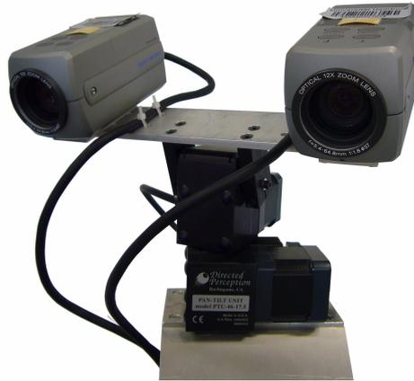
Figure 2.6.: stereo vision system mounted on a pan-tilt unit.
