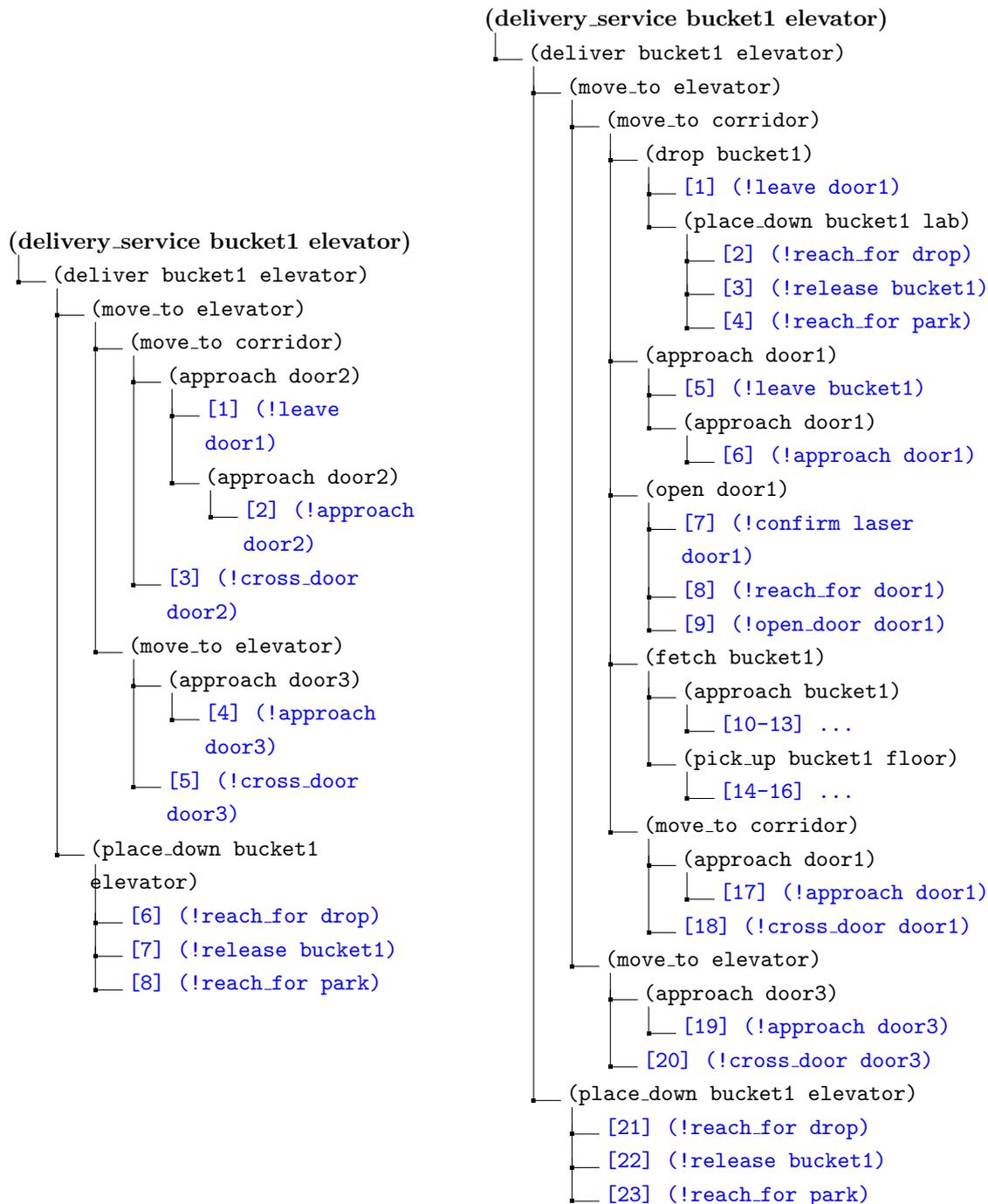
(a) Plan for delivery of the bucket with unexpectedly closed door: the revised plan let the robot cross the second door to the corridor
