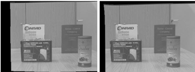
Fig. 6. Corrected and rectified pair of stereo images of a table scene. This pair of images serve as input to successive correspondance analysis procedures.
