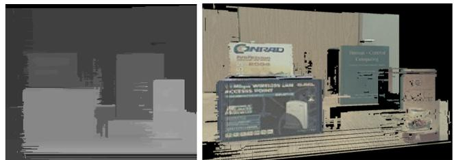
Fig. 9. Disparity map (left) based on the dynamic programming algorithm by Birchfield & Tomasi [22]. Brightness of an image point represents depth of real-world point. The brighter, the closer to the camera. A depth reconstruction (right) from the depth map is implemented by using OpenGL.
