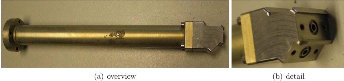
Figure 5.2: a painting gun for sealing applications
