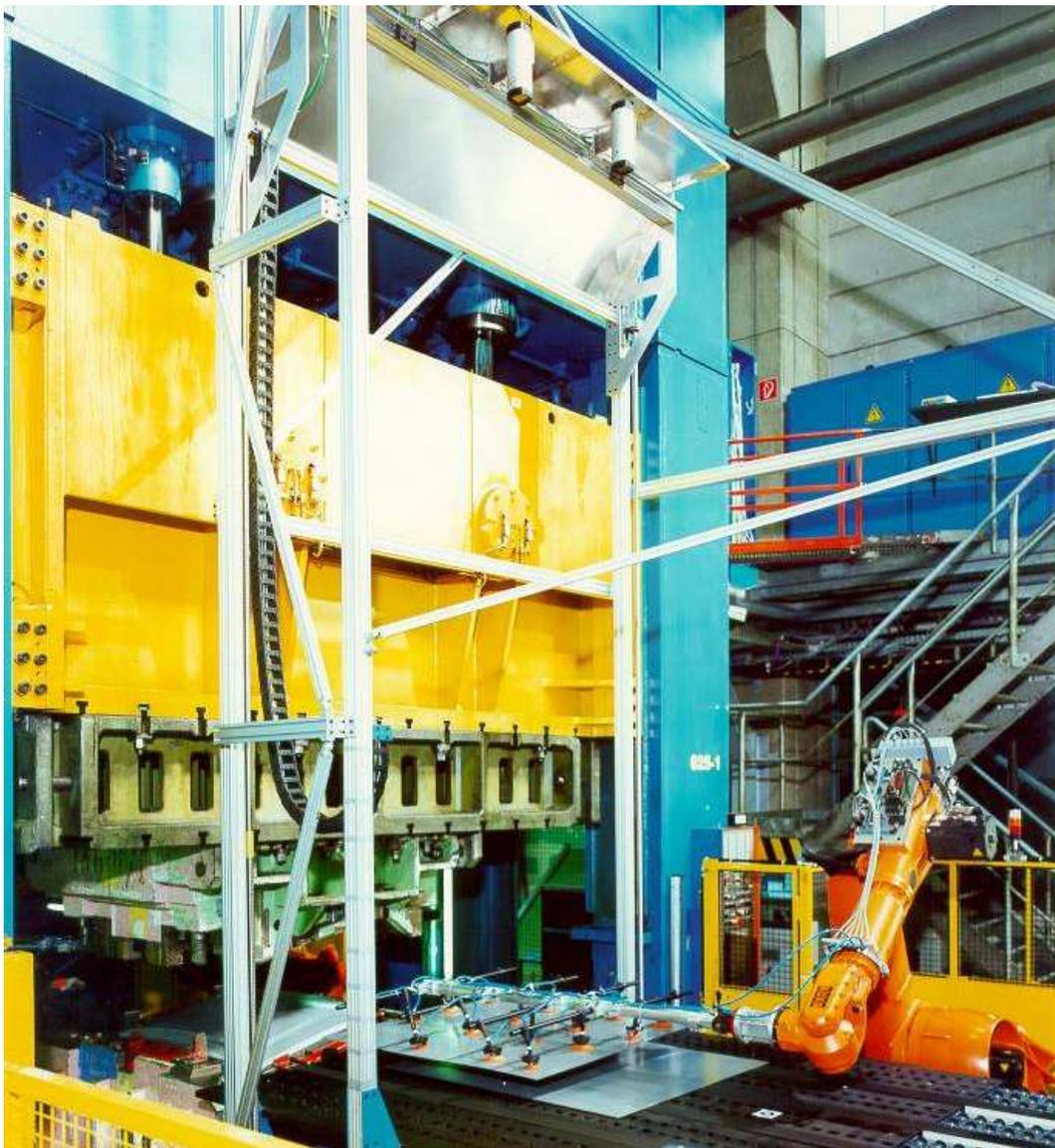
Figure 4.3: vision solution for steel sheets feeding in press shop
