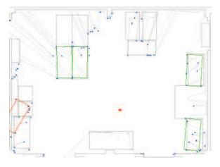
Fig. 4. Example of four correct (green) and one false (red) detected table. This is the result of the unimodal feature detector using laser range scans.
