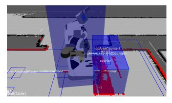
Fig. 13. Visualization of the robot's knowledge (blackboard contents) about its environment. Physical entities have a 3D bounding box and and non-physical, e.g. a placing area on a table, a 2D bounding box.
