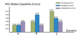
Fig. 7. RCE (Robot Capability Errors) in the ServeACoffee scenario
