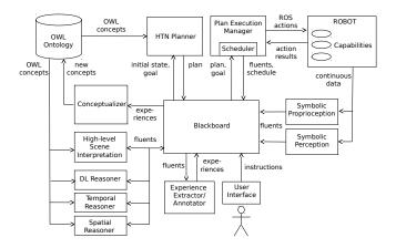
Fig. 2. The RACE Architecture contains a Blackboard as the robot's central memory. Other components mainly communicate with it in order to exchange and process Fluents.
