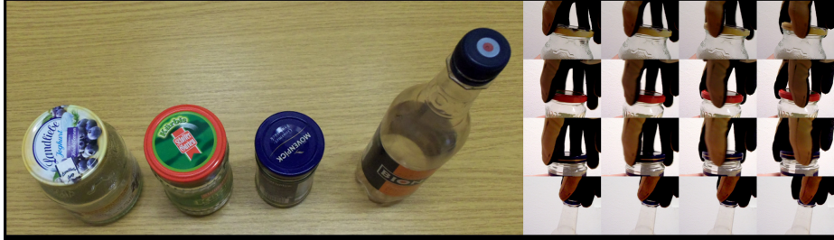
Fig. 4. Unscrewing different-sized bottle screw caps. The thumb, first, middle and ring finger participate in this scenario. Each screw cap is rotated as around 90 degree anticlockwisely, and this process is defined as a trial
