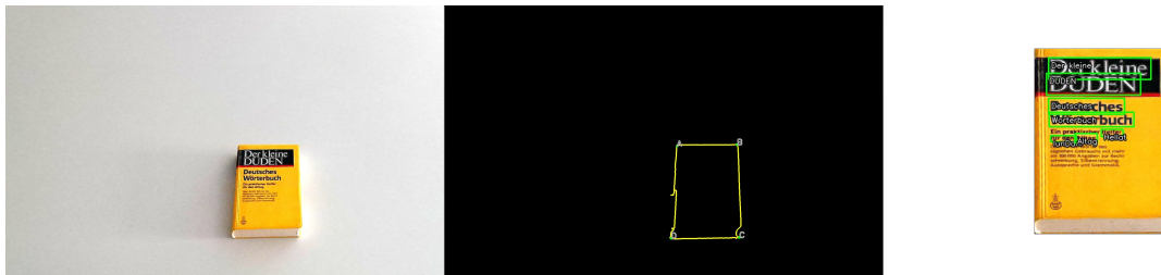
Figure 5.6: Contour also includes the side of the book. Text on the cover is still recognized
