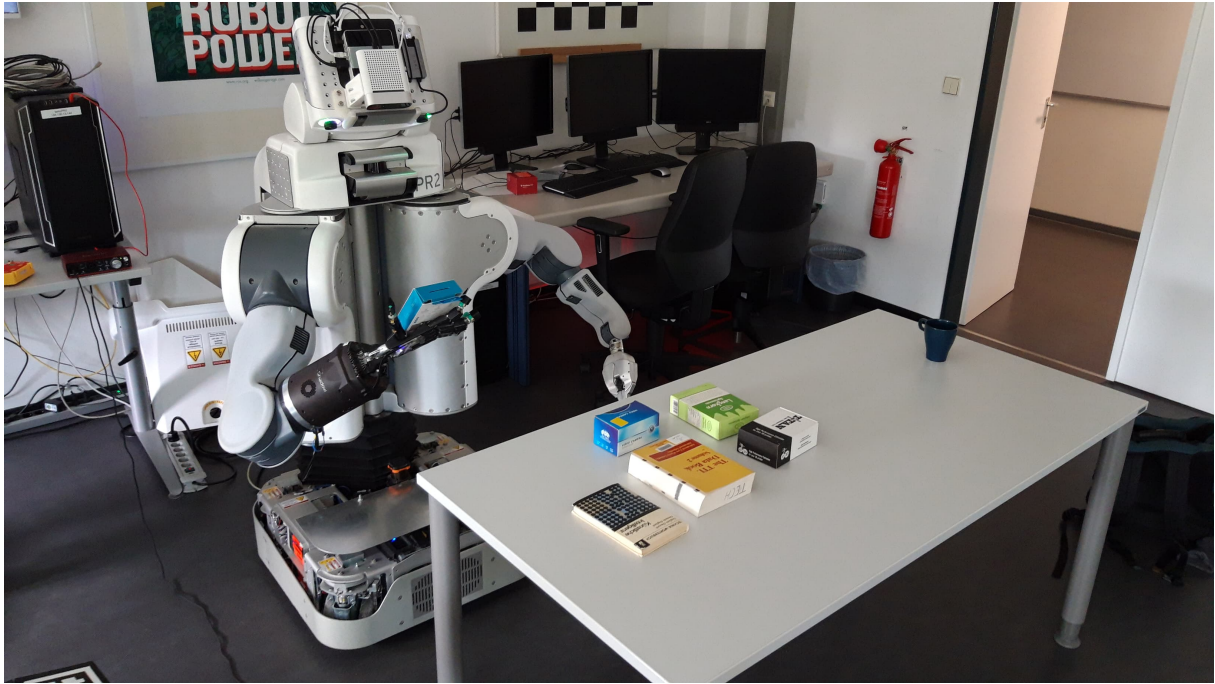
Figure 5.1: Image recording setup using the PR2 platform
