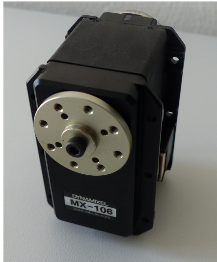
Figure 3.3.: A Dynamixel MX 106 motor is shown. At the front, the motor horn is on view. On each side, a plug for the cable is located. A bearing is located at the back.
