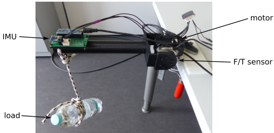
Figure 4.5.: This figure shows the experimental setup used for the analysis of the motors. The motor on the right side is clamped to the table. Attached to the motor horn on the front is a force/torque sensor. Connected to the sensor and the bearing is a lever about a bridge. At the top of the lever is an IMU on a motor control board located for velocity measurements. For applying different load to the motor, a load can be added to the front of the lever. The motor is connected to a voltage supply and controlled by the motor control board.
