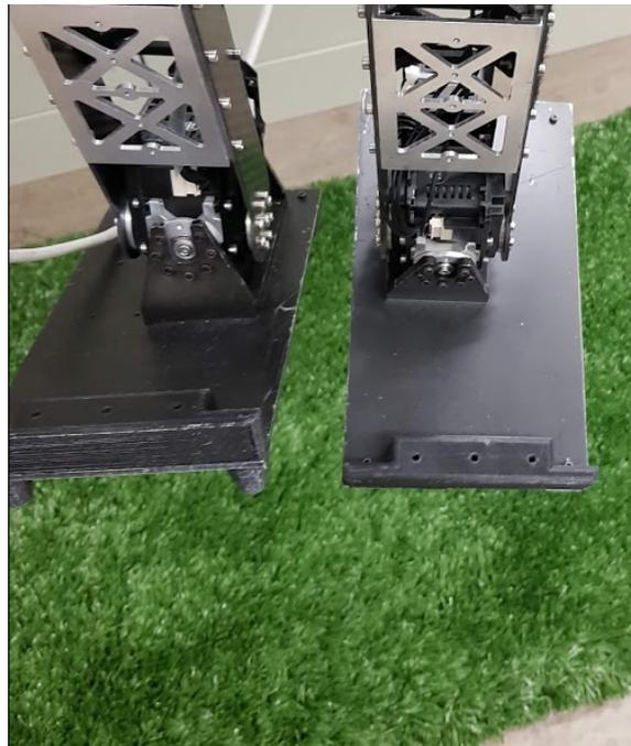
Figure 1: Feet of the Wolfgang robot made from a square aluminum base plate
