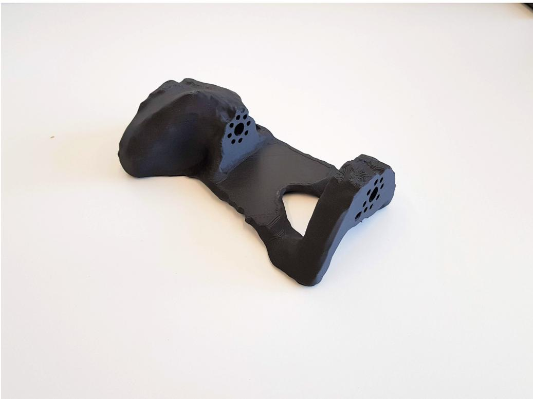
Figure 43: Printed optimized foot with screw holes of alternating depths making it impossible to mount
