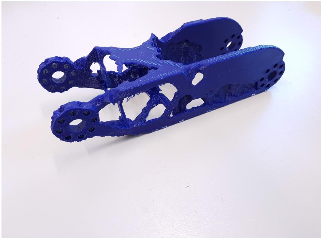
Figure 42: Printed optimized leg with support material already removed
