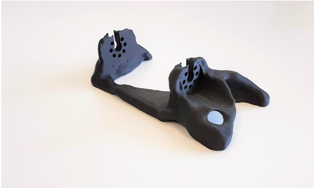
Figure 44: Optimized foot with very thin structure connecting the front and back section
