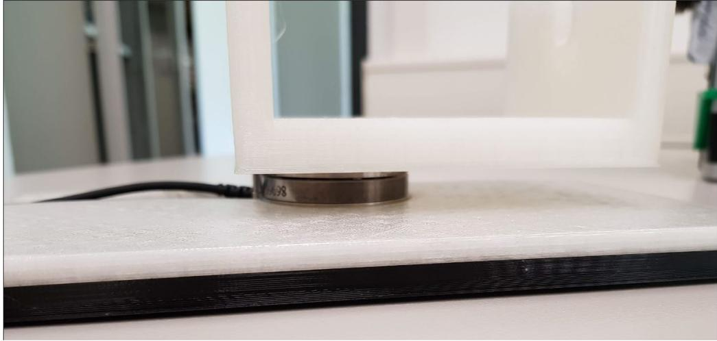
Figure 6: 3D-printed foot with closer look at an ATI Mini45 f/t-sensor connecting the top and bottom part
