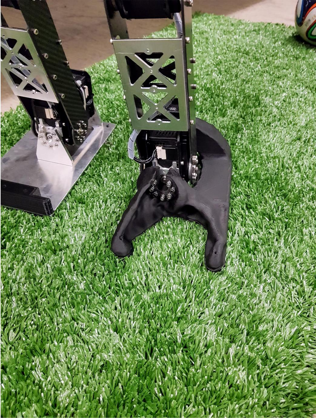
Figure 45: Optimized foot with only 15% mass retention setting mounted on the robot for a walking test
