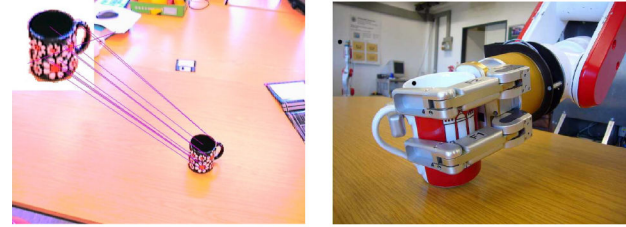
(c) Taser detects a cup using SIFT features
