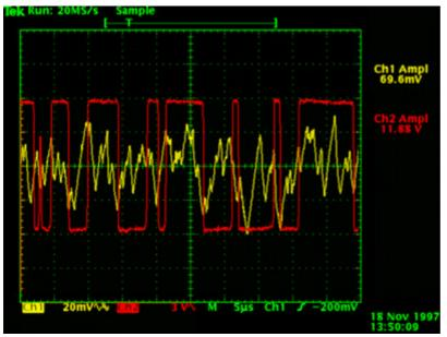
Measurement with a time scale of  $5\mu$ s/div. The picture displays 5 bits of noise at 100,000 baud. Otherwise same measurement as above.
