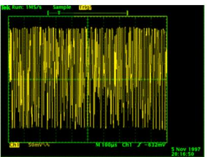
This is a picture of the output from the analog amplifier, before the signal is sampled. The time-scale is one byte/div (or ten bytes on picture) for the 100,000 baudrate.
