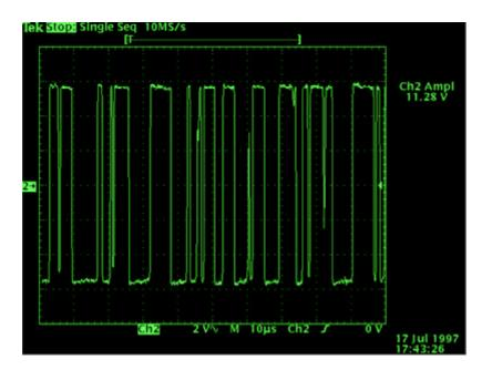
This is the output from the analog to digital converter. This picture also displays the output from the SG100 generator as observed from the computer. The UART in the computer reads the signal and assign "1" and "0" according to some (averaging) method. The time-scale is one bit/div at the maximum 100,000 baud speed.
