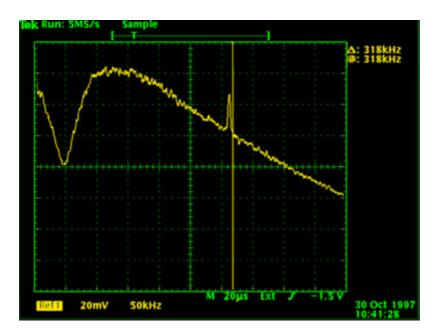
Here is the lower 500 kHz of the random signal of the diode. It is clear that, if proper amplification is used, we may actually sample the signal much faster than 100kHz. The measurement line is positioned at 318kHz, just right of one of the external signals, picked up by the measurement system. The frequency of this peak is about 312 kHz.
