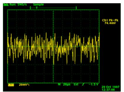
This is a measurement of the analog noise from the Zeener diode. At 20 us/div we have two bits/div at 100,000 baud. The picture displays two bytes.
