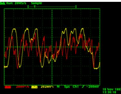
The amplitude of the input is about 0.06V (3 div). The scale of the output is about 2.9V/div (the amplitude of the analog amplifier is about 12V). The horizontal scale is 5µs/div. The picture displays 5 bits at 100,000 baud.
