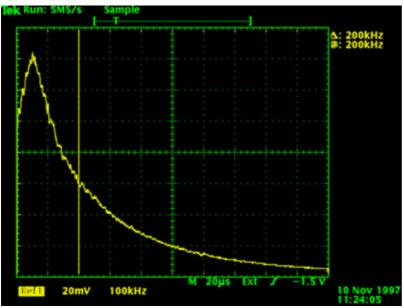
A filter (see diagram) has reduced frequencies above 100kHz, to reduce the possibility of jamming, and also to reduce the information rate of the output. It is possible, if the output looks too "noisy", that the UART of the computer refuses to read the noisy signal.
