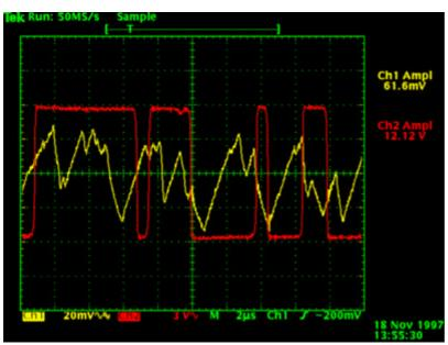
Measurement with a time scale of  $2\mu$ s/div. The picture displays 2 bits of noise at 100,000 baud. Otherwise same measurement as above.
