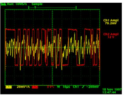
The vertical scale for the noise input (yellow) is 20mV/div, and 3V/div for the (red) output. The time scale is  $10\mu$ s/div. The picture displays 10 bits of noise at 100,000 baud.
