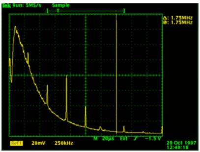
Note that a linear scale for both frequency and power has been used. The frequency scale is 250 kHz/div or 2.5MHz for the whole picture. The 0 kHz point is at the left side of the picture and the 2.5 MHz point is at the right side.
