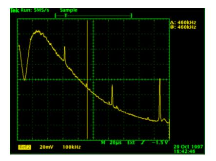
This picture is the same measurement as the one above, but with 100kHz/div. We have 1.0MHz on the whole picture. Wee see that the diode actually outputs strong signals, of all possible frequencys, up to 800kHz.
