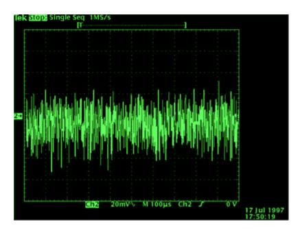
In this picture we have a time-scale of 100us/div. The picture displays the raw noise of ten consecutive bytes (at 100,000 baud).
