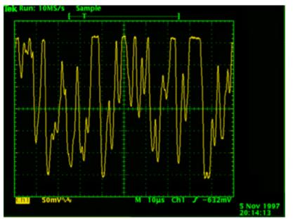
This is a picture of the output from the analog amplifier, before the signal is sampled. The time-scale is one bit/div (or one byte on picture) for the 100,000 baudrate. The output impedance is 100kOhms, at the point of measurement, and a special low capacitance probe has been used. The vertical scale is approximately 2V/div.
