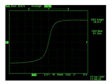
Detailed picture of the low-high transition of the digital signal. Note that no load is connected, which would make the transition much slower. It is clear that the output amplifier is very quick. Any transition time, up to 1000ns, would be acceptable.
