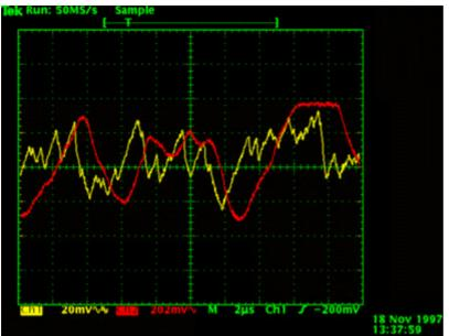
This picture have a time scale of  $2\mu$ s/div. The picture displays 2 bits at the 100,000 baudrate.
