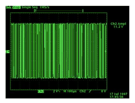
Output from the SG100 generator with a time scale of 100us/div or one byte/div. We see the stream of ten bytes.
