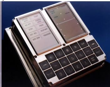
Dryden Flight Research Center EC96-43408-1. Photographed 1996 Apollo computer interface box used in the F-8 Digital Fly-By-Wire program. NASA photo by Dennis Taylor
