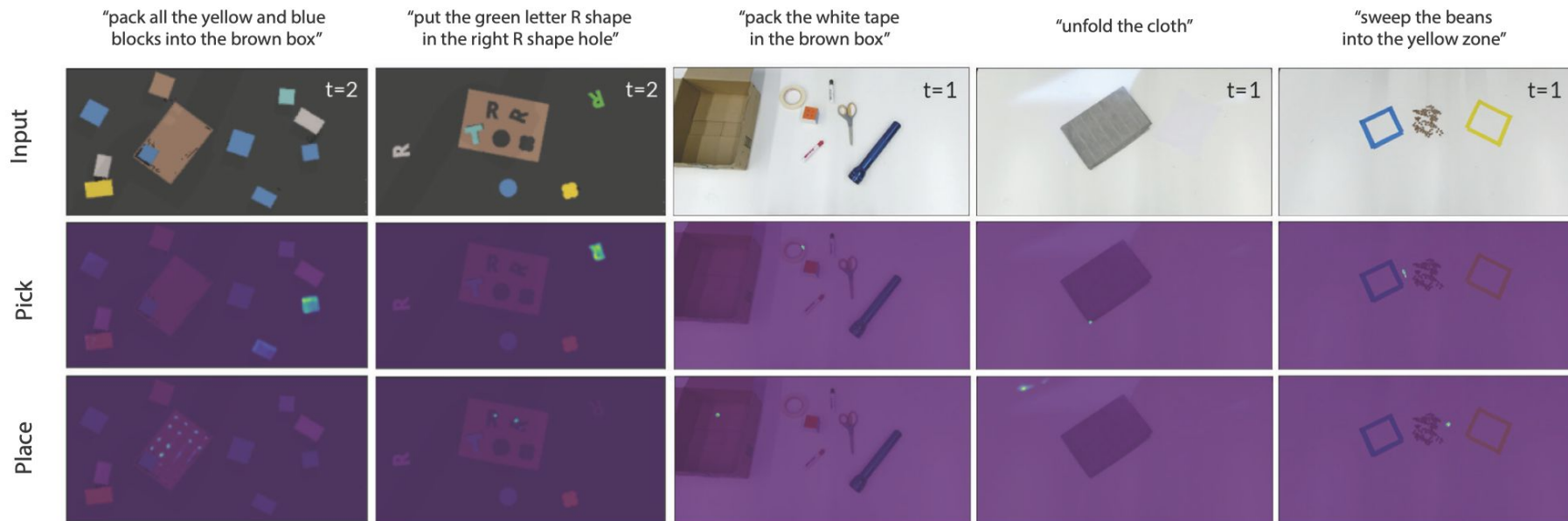
Figure 4. Affordance predictions from CLIPORT (multi) models in sim (left two) and real settings (right three). More examples in Appendix H.
