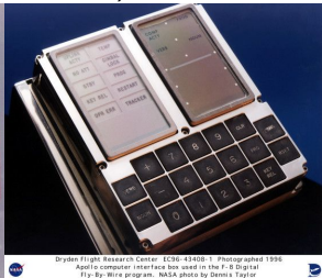
Dryden Flight Research Center EC50-43400-1 Photographed 1998 Apollo computer interface box used in the F-8 Digital Fly-By-Wire program. NASA photo by Dennis Taylor
