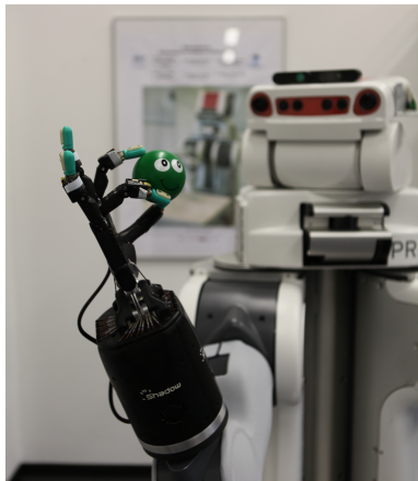
PR2 service robot with Shadow C6 electrical hand 19-DOF + 20-DOF hand
