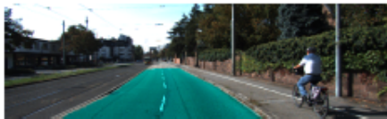
Figure: Drivable area on camera view and top view [9]
