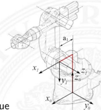
for the shown joint configuration,  $\alpha_1 = -90^\circ$  due to construction
