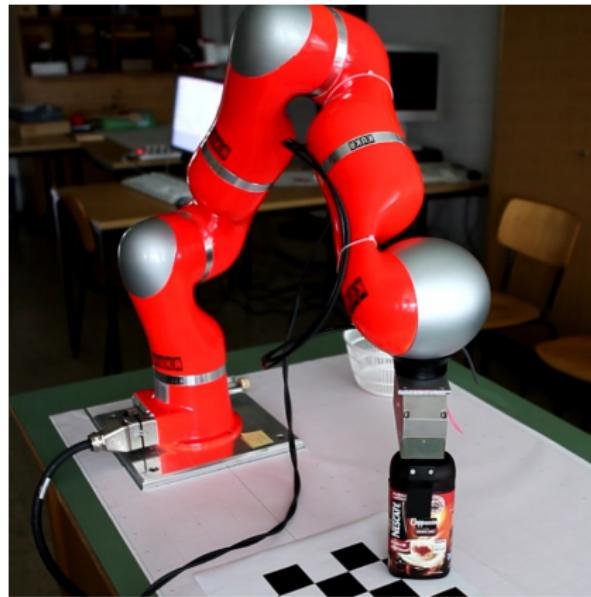
KUKA LWR 4+ arm with Schunk gripper
