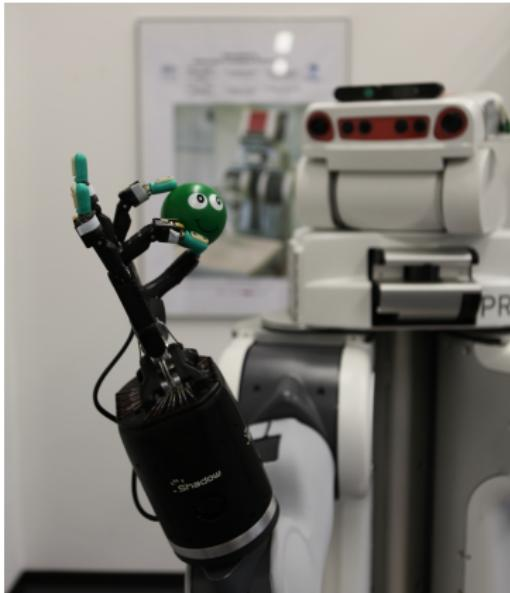
PR2 service robot with Shadow C6 electrical hand
