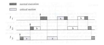
While Priority Inheritance Protocol bounds the priority inversion phenomenon, the blocking duration can still be substantial due to chain blocking. In this figure, when attempting to use its resources, J1 is blocked for the duration of two critical sections, once to wait J3 to release  $S_a$  and then to wait J2 to release  $S_b$ . This is called chain blocking.
