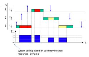
Resource ceiling for the red resource is 3. For the yellow resource, it is 2. Based on this, we can see how the system ceiling varies dynamically
