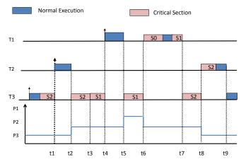
t6 : T3 unlocks S1. It awakens T1. But T3s (inherited) priority is now only P2 while P1 > C(S2) = P2. So T1 preempts T3 and runs to completion
