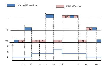
t8 : T3 unlocks S2 and goes back to its nominal priority P3. So T2 preempts T1 and runs to completion
