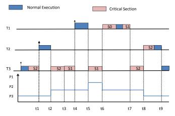
t5 : T1 can not lock S0. Currently T3 is holding S2 and S1 and C(S1) = T1 and the current priority of T1 is also P1. The (inherited) priority of T3 is now P1
