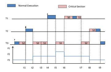
t2: T2 can not lock S2. Currently T3 is holding S2 and C(S2) = P2 and the current priority of T2 is also P2
