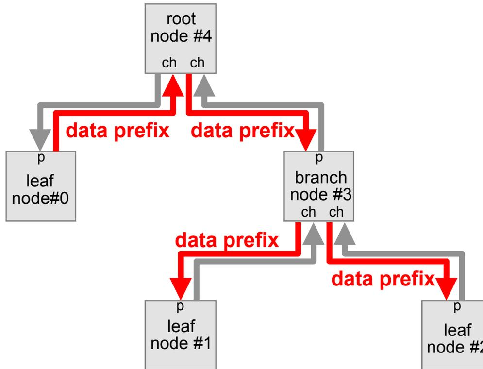
The parent of node 1 sees the data prefix and withdraws the grant, and now all nodes are correctly oriented to repeat the packet data (a "deny" is a "data prefix!") ...
