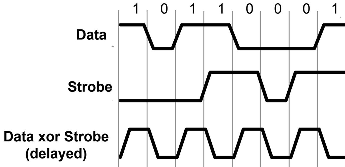
**Either Data or Strobe signal changes in a bit cell,
