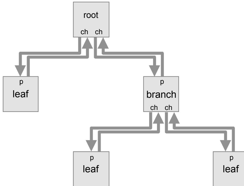
After Tree ID process, the Root node is determined and each port is labeled as pointing to a child or a parent
