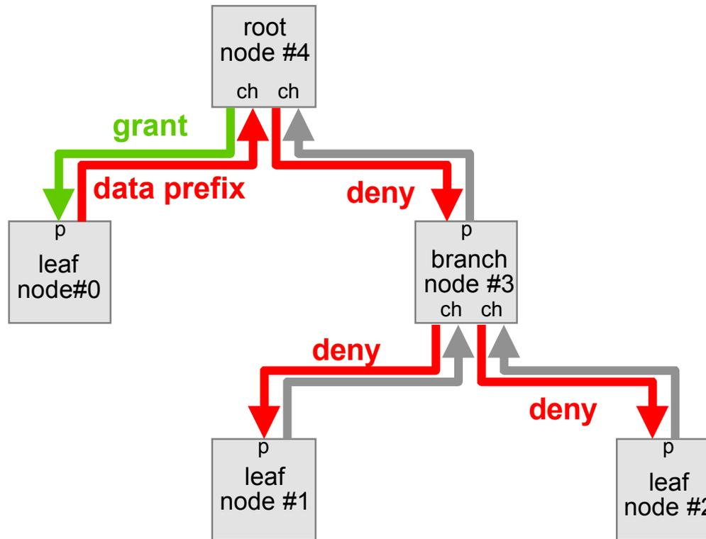
The winning node #0 changes its request to a data transfer prefix, while the losing node #2 withdraws its request ...
