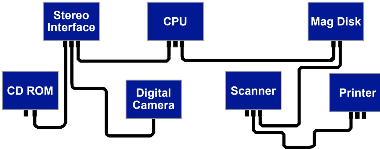
Serial Bus is “unsupervised cabling” — “non-cyclic network”; automatic address selection, no terminators, locations are arbitrary
