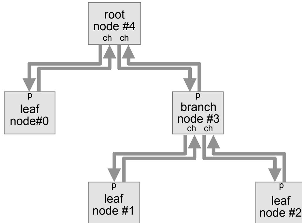
**After the self ID process, each node has a unique physical node number, and the topology has been broadcast**
