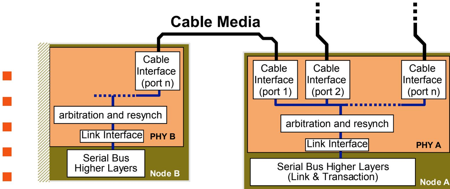
**PHY transforms point-to-point cable links into a logical bus**
