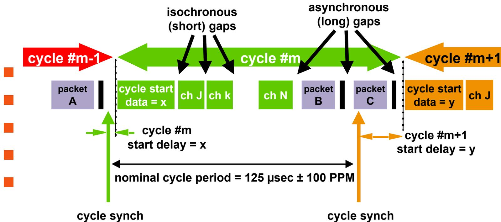
The cycle start is sent by the cycle master, which must be the root node
