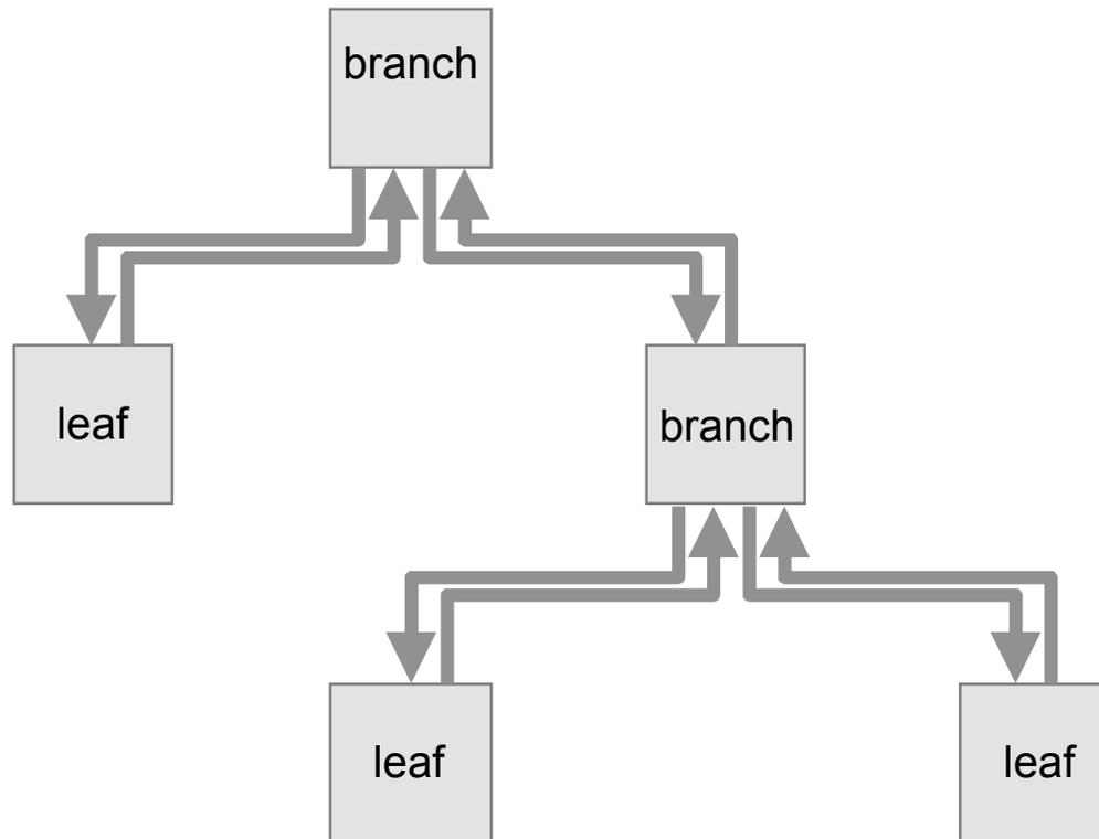
**After reset, each node only knows if it is a leaf (one connected port) or a branch (more than one connected port)**
