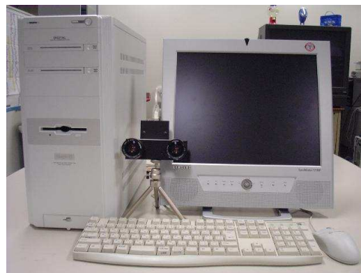
IEEE1394 High-Speed Stereo Camera, 80Hz
