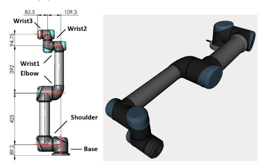
**Task 2.1 URDF description:** Create a URDF file using geometric primitives which represents the properties of the UR5. Use the pose in the right picture above as the zero positions for your joints. Visualize the arm in the visualization tool (rviz) to verify your URDF description and show your result to a supervisor.
