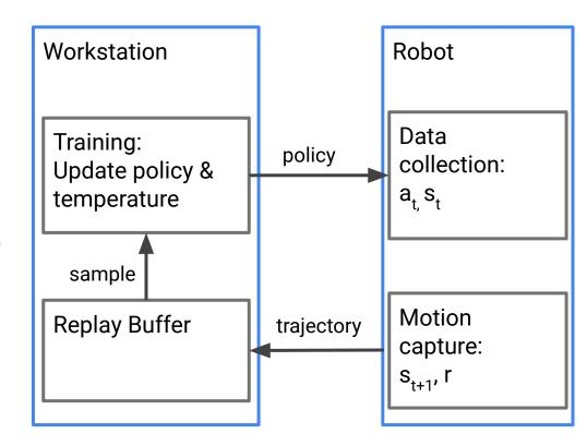
Approach 2: Data Efficient Reinforcement Learning for Legged Robots
