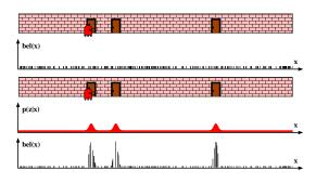
Random initialization. Incorporation of the motion model with weighting of the samples.
