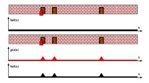
Convolution of prior with motion model followed by incorporation of the measurement model.
