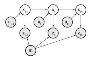
Map m, measurements z and controls u are known, robot pose x must be inferred
