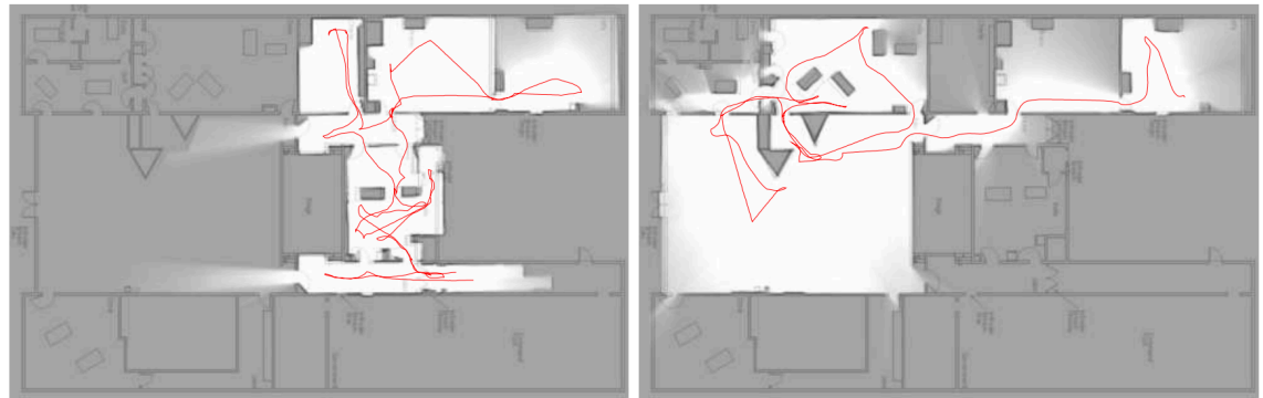
Individual maps from two robots using single-Robot SLAM algorithm [2]
