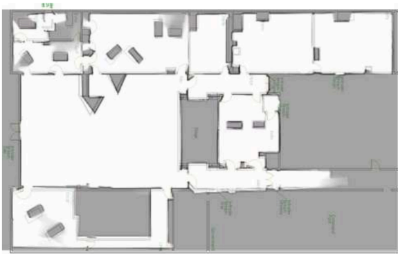
Combined map using multi-Robot SLAM algorithm [2]
