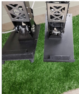
Feet of the robot made out of aluminum and carbon
