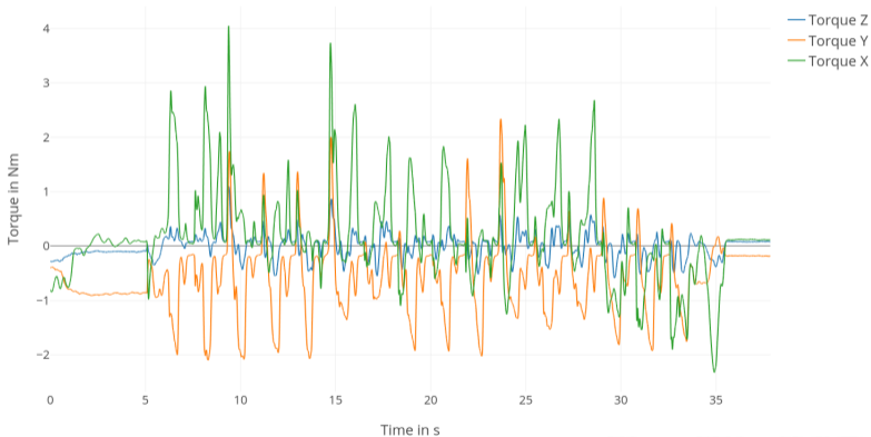
Graph showing torques in x-,y- and z-direction reported by the ATI Mini45 f/t-sensor
