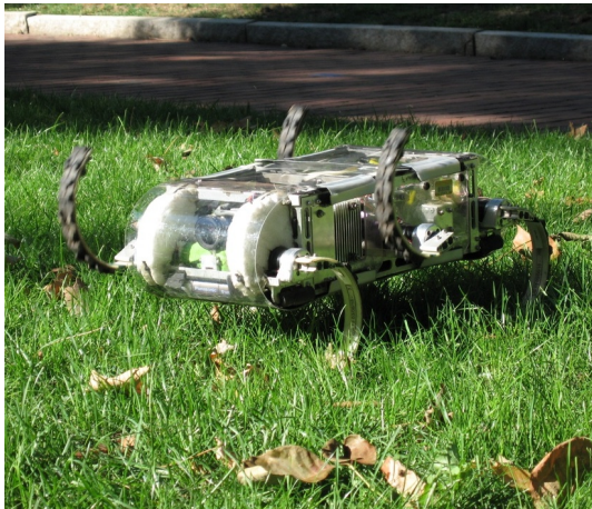
Figure: Example of a hexapedal robot with static balance [Lopes, 2008]
