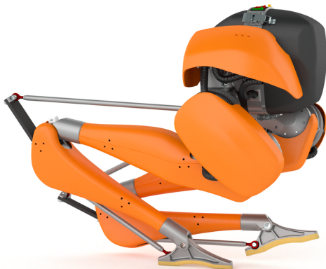
Figure: Side view of the Robot Cassie from Agility Robotics [Shelton et al., 2017]
