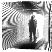
Point clouds created by rotated line scanners. [2, p. 46, fig. 2.21]
