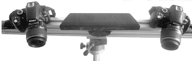
Rotated stereo-camera rig and a Kinect. [6, p. 5, fig. 1.2]
