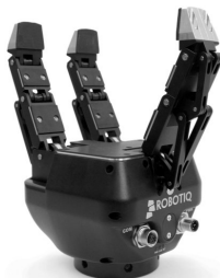
Figure: A 3-finger gripper. Retrieved from https://robotiq.com/products/3-finger-adaptive-robot-gripper (last checked 01.11.2017)
